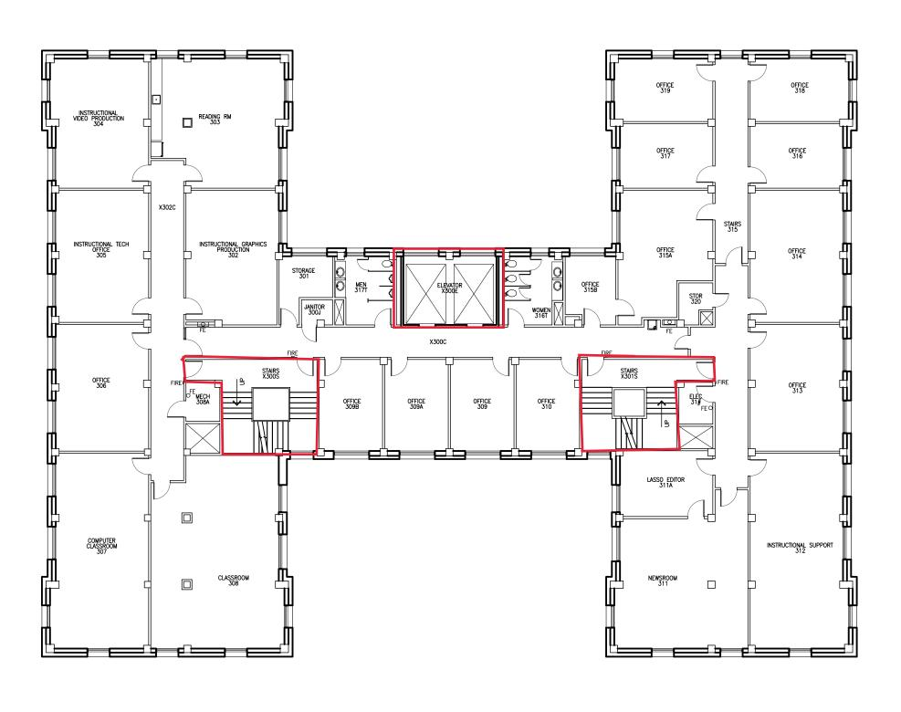
Key:Firewall: all penetrations must be firestopped All penetrations into floors must be firestopped
