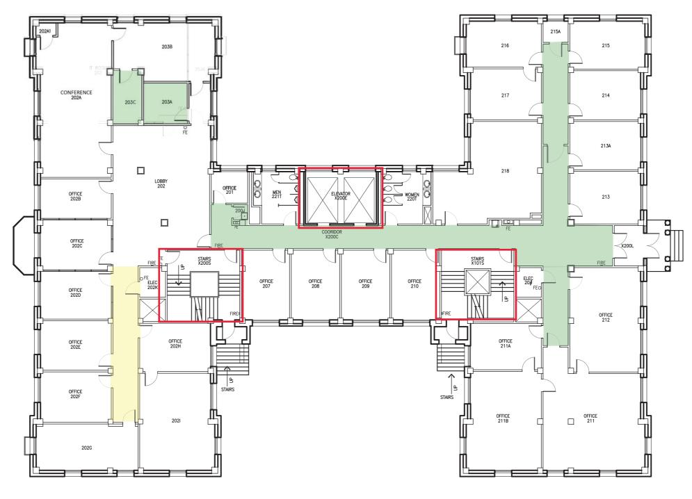
Key:Firewall: all penetrations must be firestopped All penetrations into floors must be firestopped
