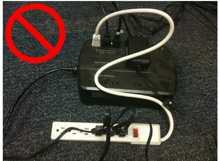
Improper "daisy-chained" power strip/UPS: Power strips/UPSs must be plugged directly into an outlet.
