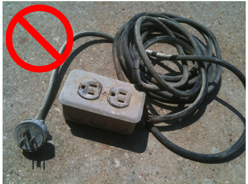
Prohibited extension cord: cord is not UL-listed and is cracked/damaged.
