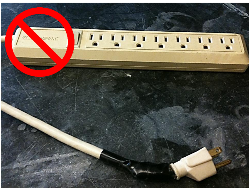
Damaged power strip: insulation has pulled out of plug. This should be disposed of immediately.
