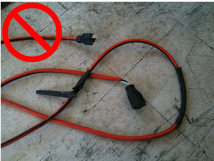
Extension cord damaged: insulation has pulled out of plug, cord is taped in several locations, and ground prong is missing. This should be disposed of immediately.
